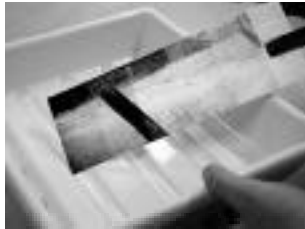
A test strip lets you choose the best exposure for your print.
